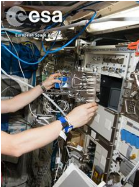
Installation of the Experiment Interface Extension featuring an MKS Mass Flow Controller for the PK-4 Plasma Crystal Laboratory on the International Space Station
