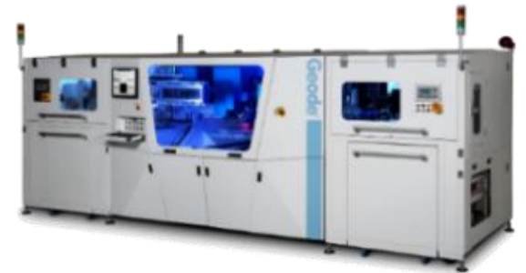
Geode: Via drilling for HDI PCB
